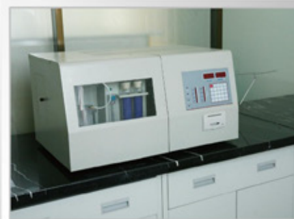
Fast intelligent sulfur determination instrument
